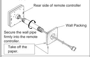
Slide the box nut over the remote controller wires and screw it onto the wall pipe.
