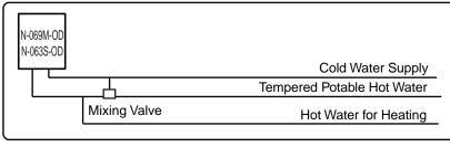
For Space Heating Purposes: If the system requires water for space heating at a higher temperature than for other uses, means such as a mixing valve shall be provided to temper the water for the other uses to help prevent scalding.
